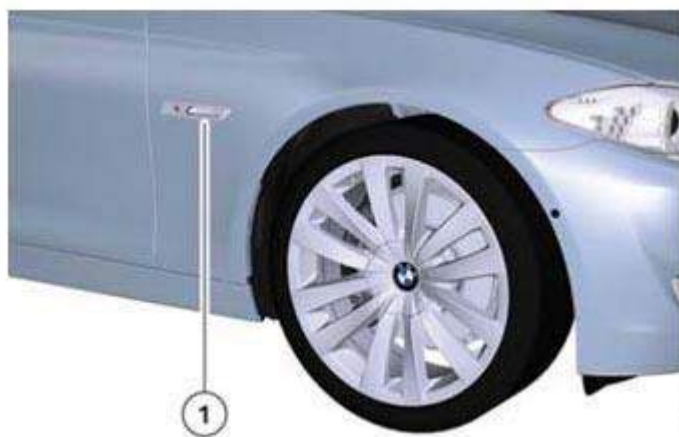
Fig. 10: Identifying F10 Installation Location Of Parking Assistant Ultrasonic Sensor In Side Marker
