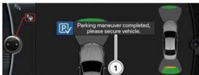
Fig. 25: Identifying F10 Parking Assistant Completion Of Parking Process Courtesy of BMW OF NORTH AMERICA, INC.
