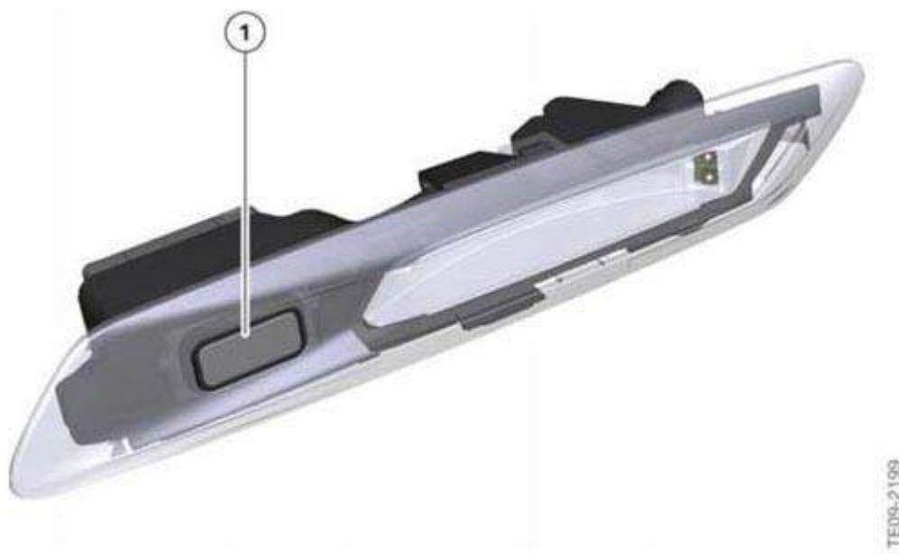
Fig. 11: Identifying F10 Parking Assistant Ultrasonic Sensor In Right Side Marker Turn Signal Indicator Courtesy of BMW OF NORTH AMERICA, INC.
