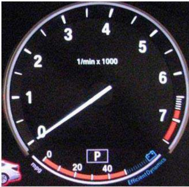
Fig. 3: Identifying F10 Current Fuel Consumption Display In Coasting (Overrun) Mode Courtesy of BMW OF NORTH AMERICA, INC.
