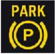
Fig. 15: Identifying F10 Indicator Light, Parking Brake Fault Display Courtesy of BMW OF NORTH AMERICA, INC.
