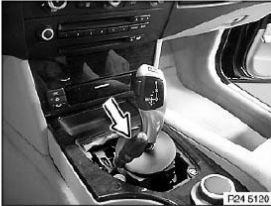
Fig. 74: Releasing Transmission Lock Courtesy of BMW OF NORTH AMERICA, INC.
