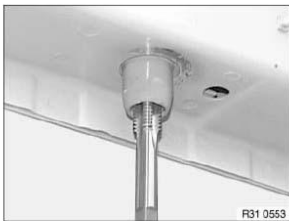
Fig. 8: Applying Thread For Heli-coil Thread Courtesy of BMW OF NORTH AMERICA, INC.
