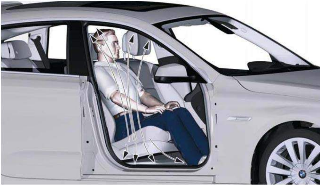
Fig. 5: Measuring Procedure Of CIS Mat Courtesy of BMW OF NORTH AMERICA, INC.
