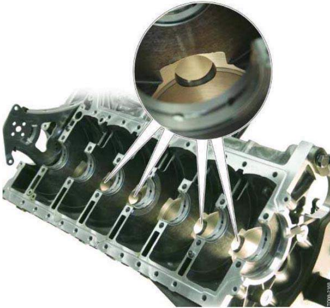
Fig. 5: Identifying Ventilation Holes In Crankcase - N55 Courtesy of BMW OF NORTH AMERICA, INC.
