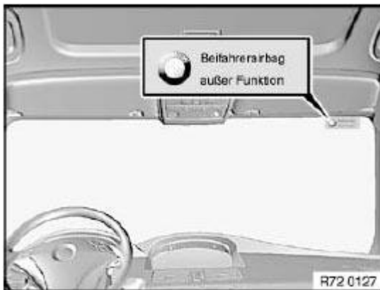
Fig. 45: Locating Warning Sign, Passenger Airbag Label Courtesy of BMW OF NORTH AMERICA, INC.
