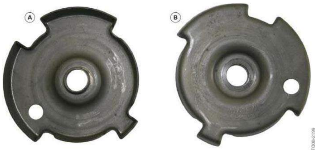
Fig. 28: Identifying Camshaft Sensor Wheel (Rear And Front View) - N55 Courtesy of BMW OF NORTH AMERICA, INC.
