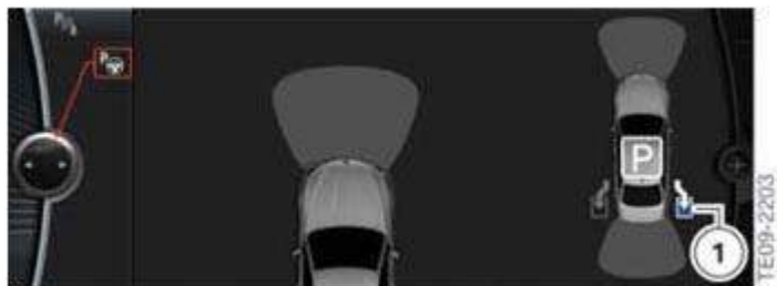
Fig. 17: Identifying F10 Parking Display (Parking Assistant Is Not Activated, With Parking Space Found To Right)
