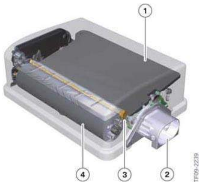
Fig. 37: F10 Structure Of Sensor For ACC Stop & Go Courtesy of BMW OF NORTH AMERICA, INC.
