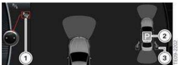
Fig. 16: Identifying F10 Parking Display With Parking Assistant Activated Courtesy of BMW OF NORTH AMERICA, INC.
