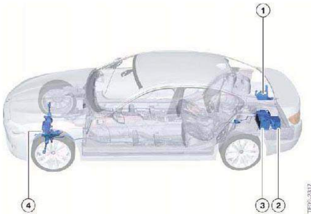
Fig. 28: Identifying F10 24V Battery Charging Components And Line Routing Courtesy of BMW OF NORTH AMERICA, INC.
