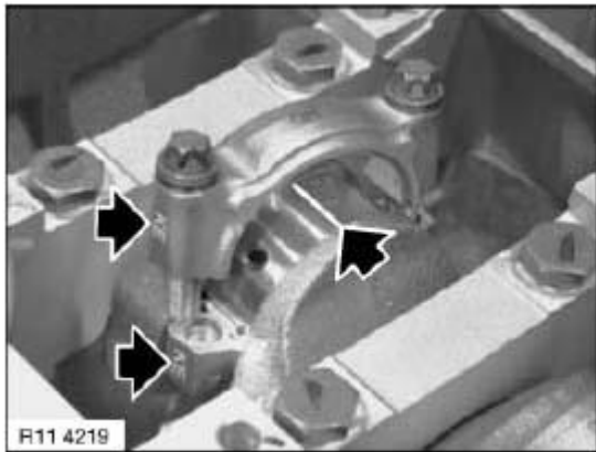
Fig. 129: Locating Conrod Bearing Clearance Courtesy of BMW OF NORTH AMERICA, INC.
