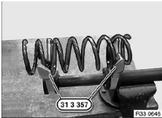
Fig. 102: Identifying Special Tools 31 3 357 Onto Coil Spring Courtesy of BMW OF NORTH AMERICA, INC.
