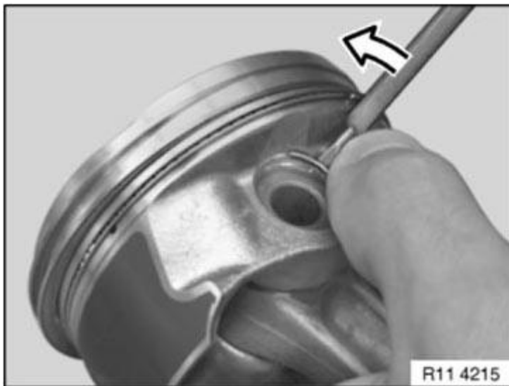
Fig. 176: Removing Retaining Ring From Piston Courtesy of BMW OF NORTH AMERICA, INC.
