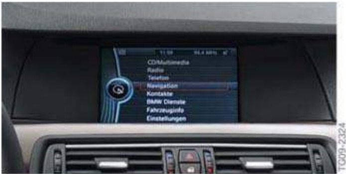
Fig. 6: Identifying F10 CID With 7 Screen Diagonal Courtesy of BMW OF NORTH AMERICA, INC.
