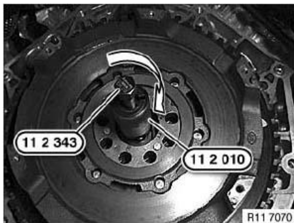
Fig. 121: Identifying Special Tool (11 2 010) And (11 2 343) Courtesy of BMW OF NORTH AMERICA, INC.
