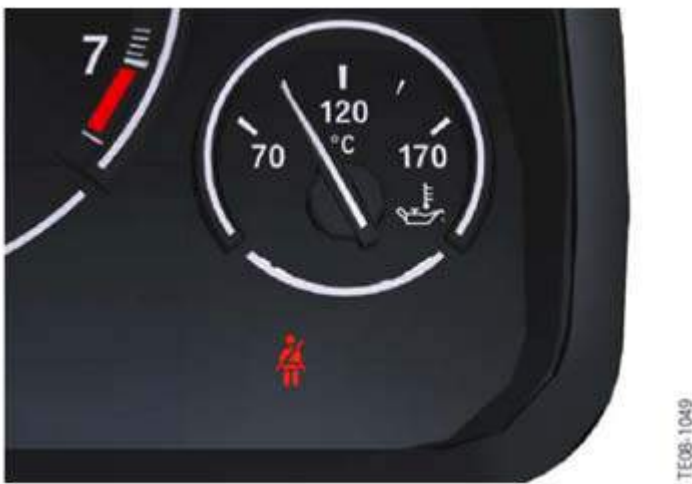
Fig. 25: Display Seat Belt Warning Light Courtesy of BMW OF NORTH AMERICA, INC.
