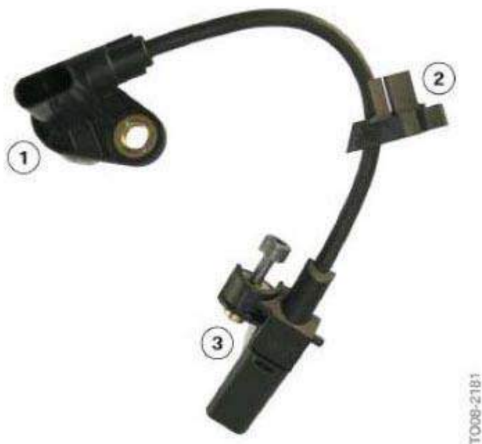
Fig. 66: Identifying Crankshaft Sensor With Multipole Sensor Wheel - N55 Courtesy of BMW OF NORTH AMERICA, INC.
