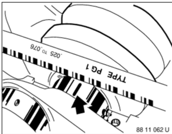
Fig. 115: Measuring Main Bearing Clearance
