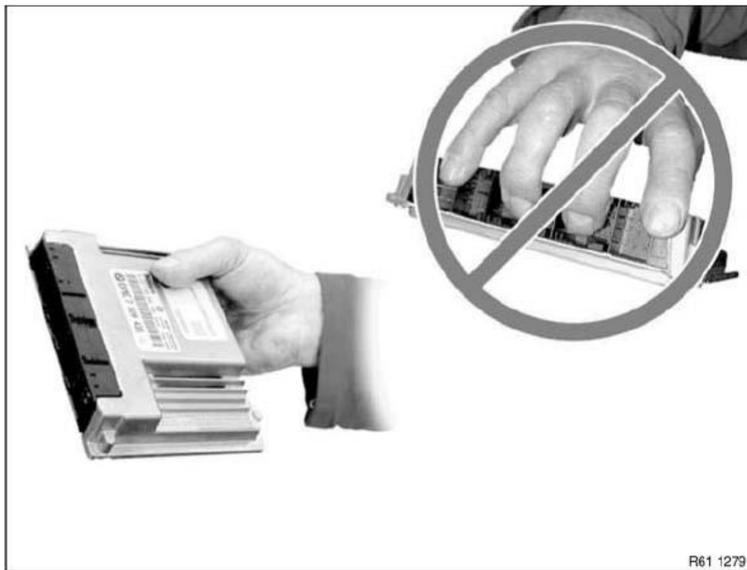
Fig. 266: Precaution For - Do Not Touch Pins Or Multi-Pin Connectors Directly Courtesy of BMW OF NORTH AMERICA, INC.
