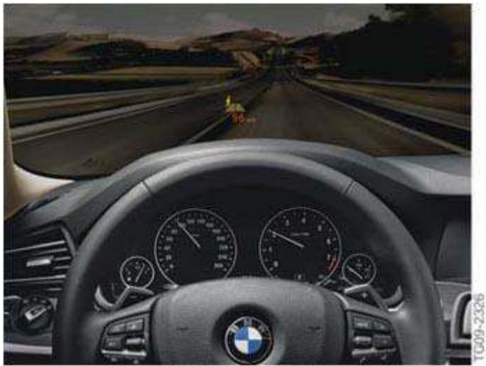
Fig. 8: Identifying F10 Night Vision Display In Head-Up Display Courtesy of BMW OF NORTH AMERICA, INC.
