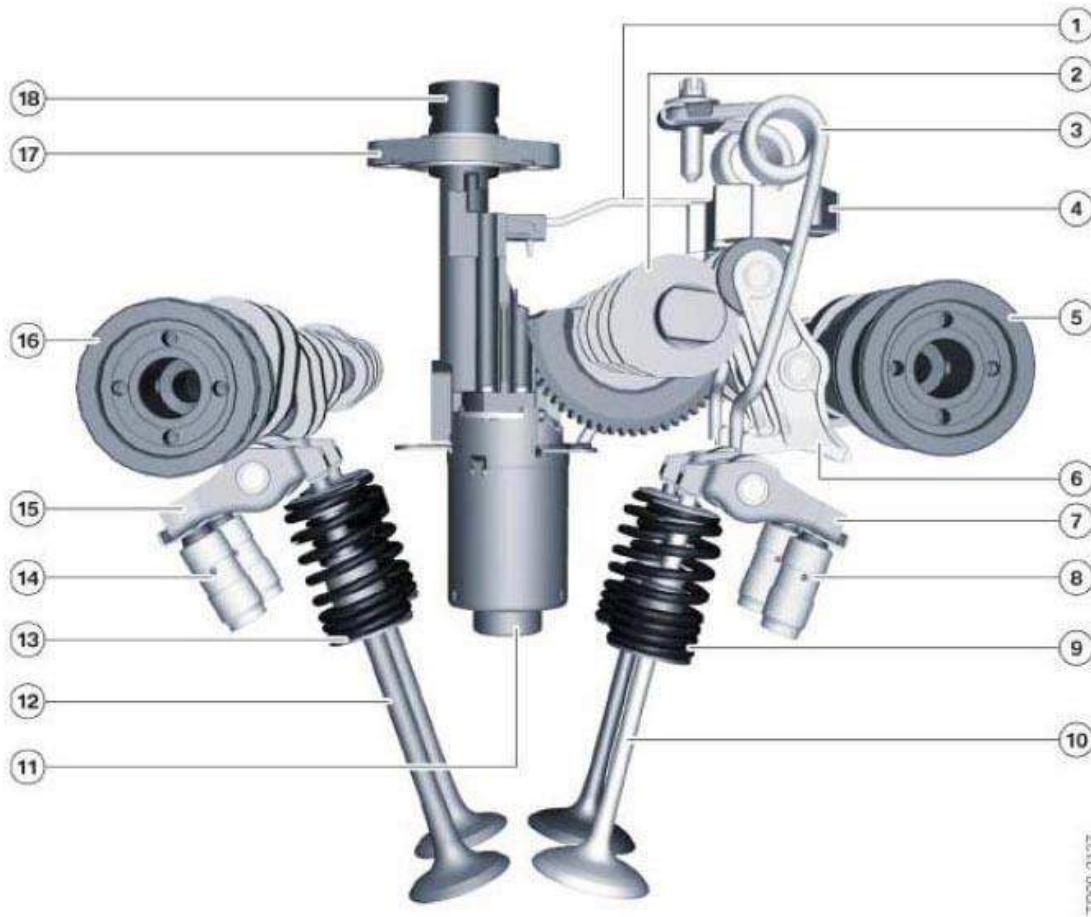
Fig. 33: Design Of Valve Lift Adjustment - N55 Courtesy of BMW OF NORTH AMERICA, INC.
