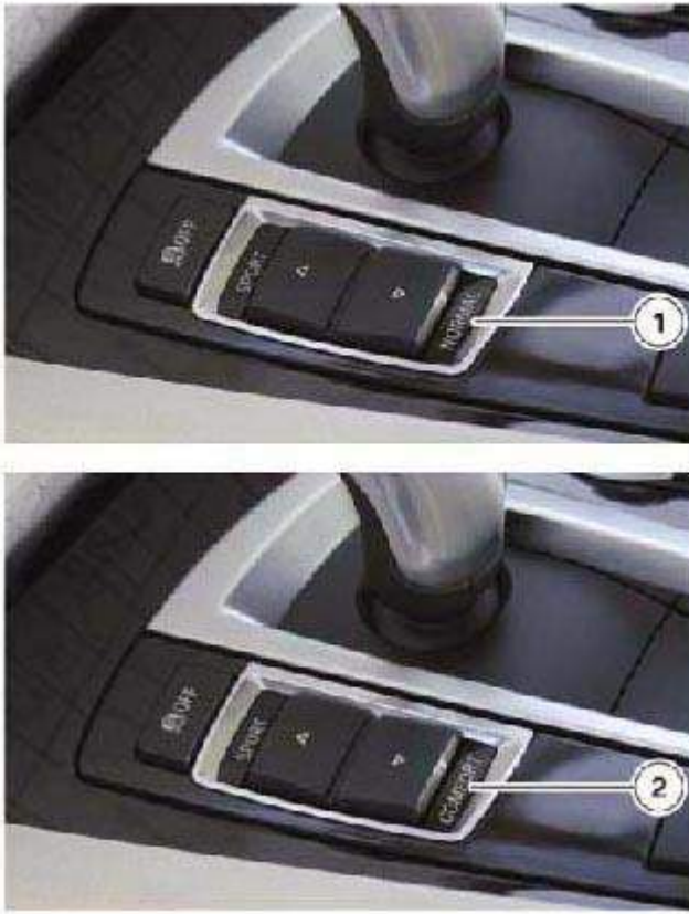
Fig. 33: Identifying F10 Driving Dynamics Control Switch Courtesy of BMW OF NORTH AMERICA, INC.
