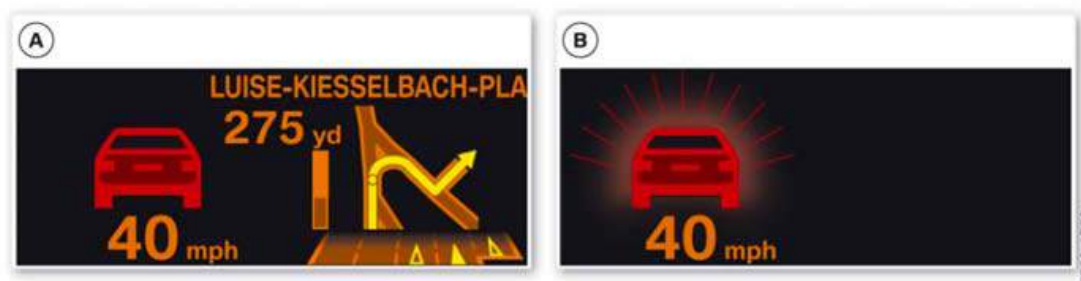
Fig. 43: Identifying Collision Warning In Head-Up Display
