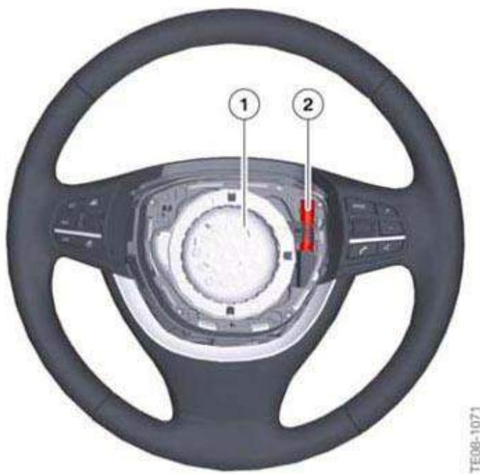
Fig. 15: Identifying Vent Valve And Gas Generator On Steering Wheel
